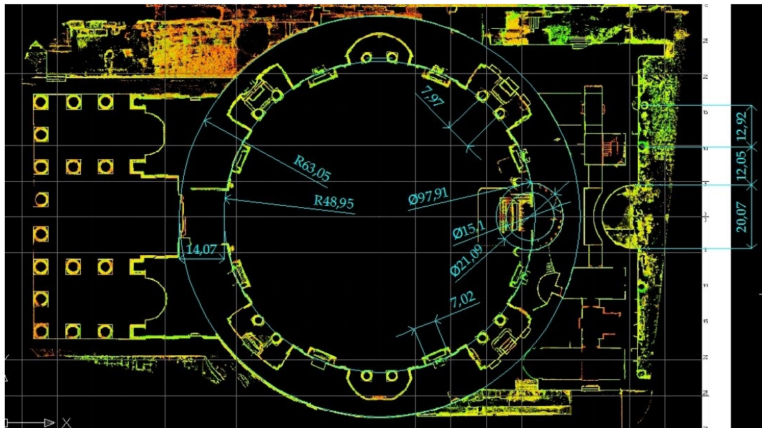
Pic.9. Dimensions of the Pantheon plan in Roman cubit ( Analysis of laser measurements from http://www.digitalpantheon.ch/ ).
